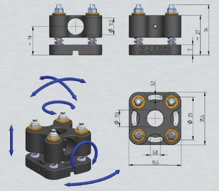
**HX-11**Very precise plastic disc spring bracket for laser modules with Ø 11mm.
